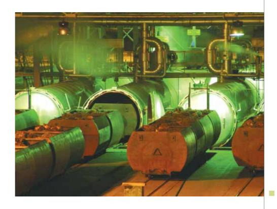
The process consists of sterilisation, separation, soaking, extraction of the oil from the pulp, clarification and recovery of the kernels from the bagasse. Two products are obtained from the palm kernel: palm kernel oil and palm kernel meal, the latter being a highly valuable source of animal feed.
