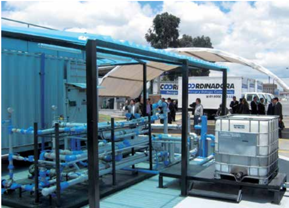
Biofuel storage and blend station during the long-term testing with oil palm biodiesel in a fleet of cargo trucks.
