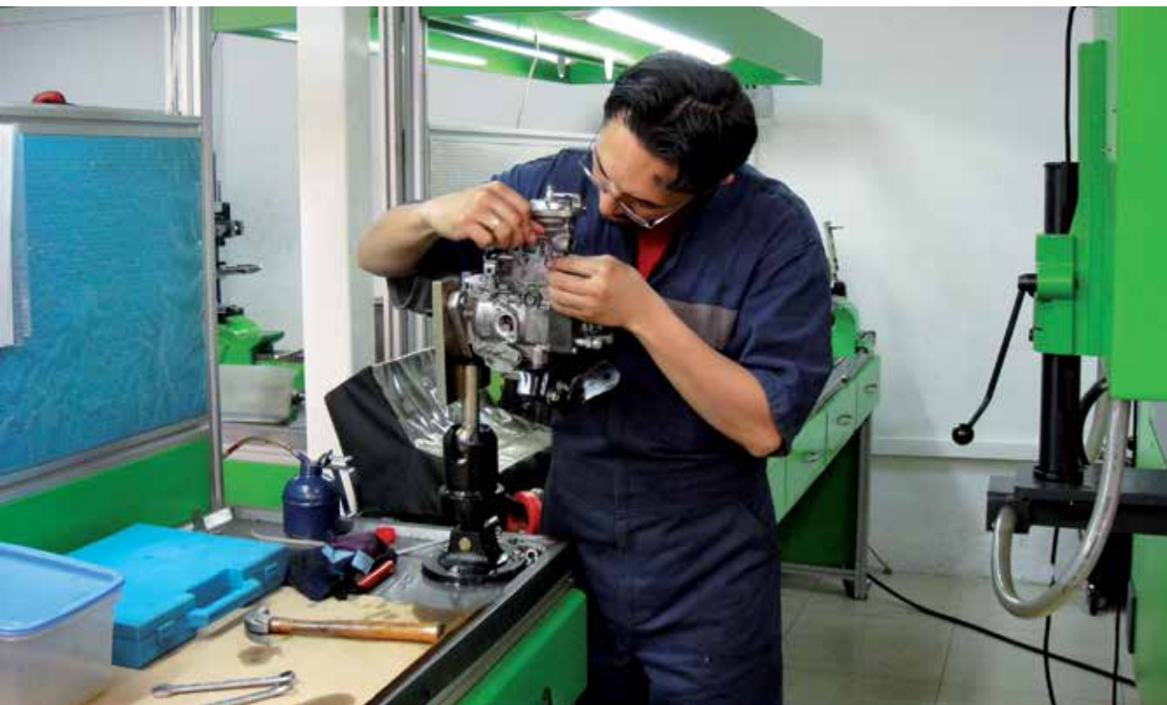
Mechanical check of the injection system in Chevrolet NKR3 vehicles.
